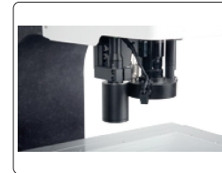
spectral confocal sensor ( optional ), thickness of glass or plastic film can be measured according to the refractive index, measuring accuracy is 5µm
